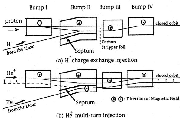
Figure.2 Comparison of Booster Injections for Negative and Positive Ions
