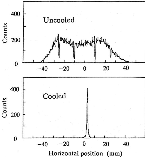
Figure 5. Horizontal beam profiles for (a) uncooled and (b) cooled 85-MeV  $N^{5+}$  beams. The dips in the profile result from the shadows of 1-mm thick wires, which are inserted to calibrate the beam position.
