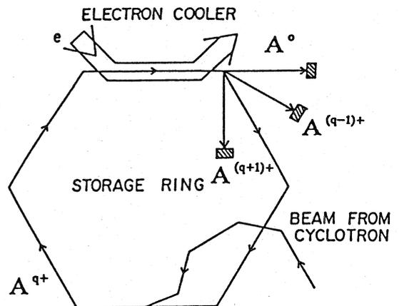
Figure 7. Schematics of the storage ring, the electron cooler and the detection system of charge-changed particles.
