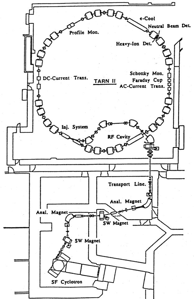
Figure 1. Schematic diagram of TARNII and injector SF cyclotron.
