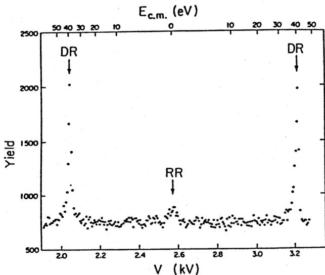
Figure 8. Yield of neutral He atoms formed in the electron cooler as a function of the electron acceleration voltage. The c.m. energy scale is also shown. The maxima on the both sides correspond to DR, while the bump on the center is due to RR.
