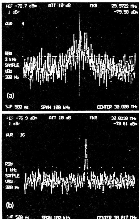
Figure 3. Frequency spectra of longitudinal Schottky signals for (a) uncooled and (b) cooled 20-MeV proton beams.
