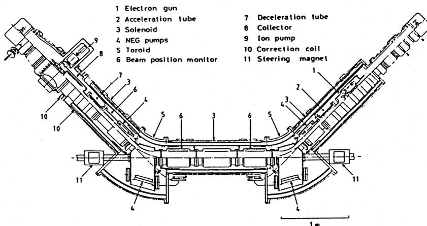
Figure 2. Layout of electron cooling device.
