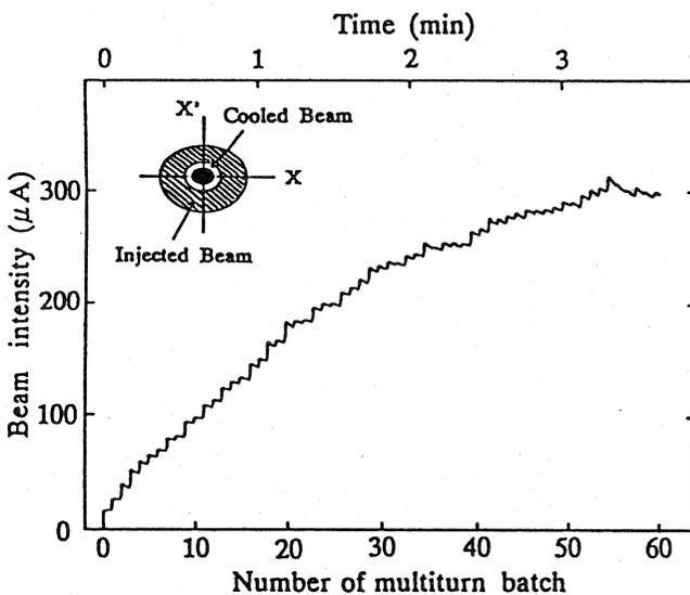
Figure 6. Intensity increase during cool stacking as a function of the number of multiturn batches. The inset shows schematically represented phase spaces for the cooled and stacked beam and for the multiturn injected beam.
