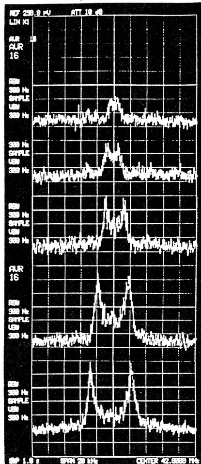
Figure 4. Splitting of frequency spectrum of Schottky signal with increase in stored beam intensity (16-MeV p). From the top, intensities of proton beam are 3, 7, 16, 54 and 90  $\mu$ A.
