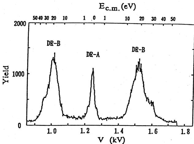
Figure 10. Yield of neutral He+H atoms formed in the dissociative recombination  $\text{HeH}^+ + e \rightarrow \text{He} + \text{H}$  as a function of electron acceleration voltage. The c.m. energy scale is also shown. The time window is 0.92-1.47 s and the electron current is 0.2 A
