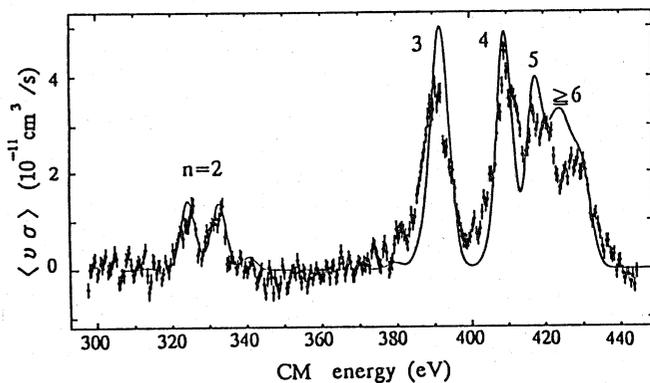
Figure 9. DR spectrum of He-like nitrogen ions in their ground state:  $\text{N}^{5+}(1s^2)+e \rightarrow \text{N}^{4+}(1s2lnl') \rightarrow \text{N}^{4+}(1s^2nl') + h\nu$ . The data are compared to the preliminary calculations by N.R.Badnell folded with the electron velocity distribution for  $kT_{\perp} = 0.5$  eV and  $kT_{\parallel} = 0.005$  eV.
