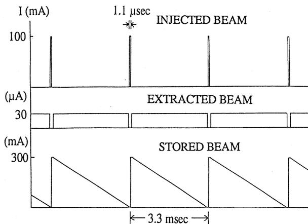
Fig.4 Conversion of the pulsed beam to a continuous beam and the intensity of the stored beam.
