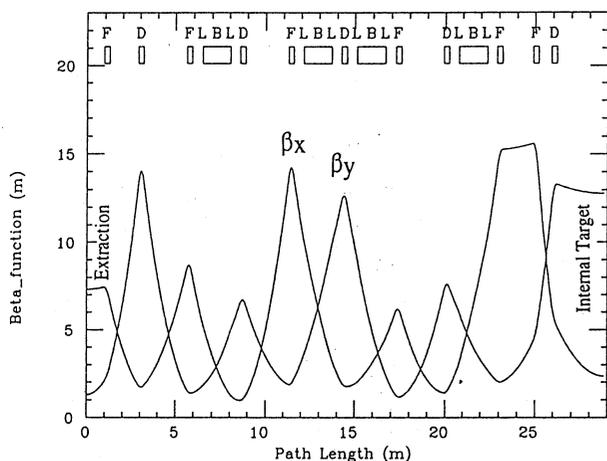
Fig.2 Betatron function of a quarter of the ring in the booster-storage mode.
