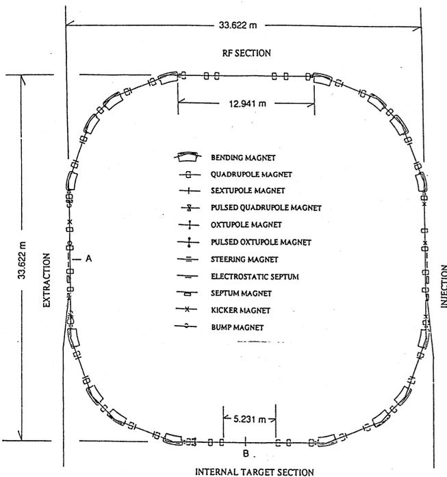
Fig.1 Structure of the stretcher-booster ring.
