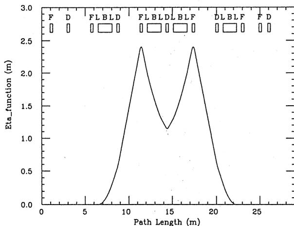
Fig.3 Off-energy function in the booster-storage mode.
