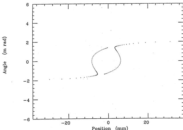
Fig.5 Trajectory of a resonating electron in horizontal phase space at the electrostatic septum in the half-integer resonance extraction.
