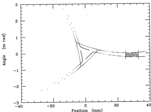
Fig.6 Trajectory of a resonating electron in the achromatic extraction mode. Emittance of the extracted beam is improved to 0.06 mm mr by bump magnets.
