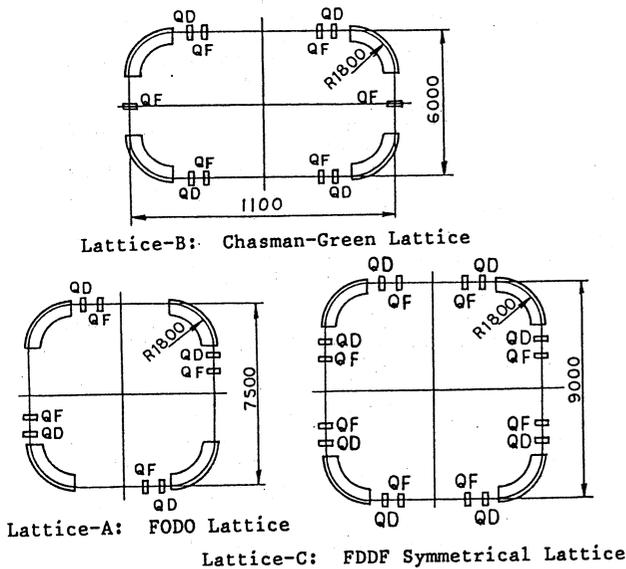
Fig. 1 Schematic layouts of considered lattices
