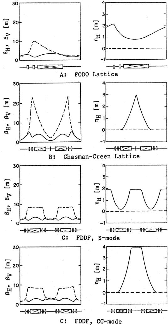
Fig. 2 Betatron functions and Dispersion functions (—: Horizontal, ----: Vertical)
