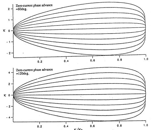
Fig.2 Eigen-tunes vs. tune depression  $\kappa_s/\kappa_0$  in the cubic-force approximation
