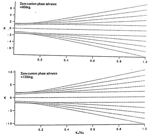
Fig.1 Eigen-tunes vs. tune depression  $\kappa_s/\kappa_0$  in the linear-force approximation
