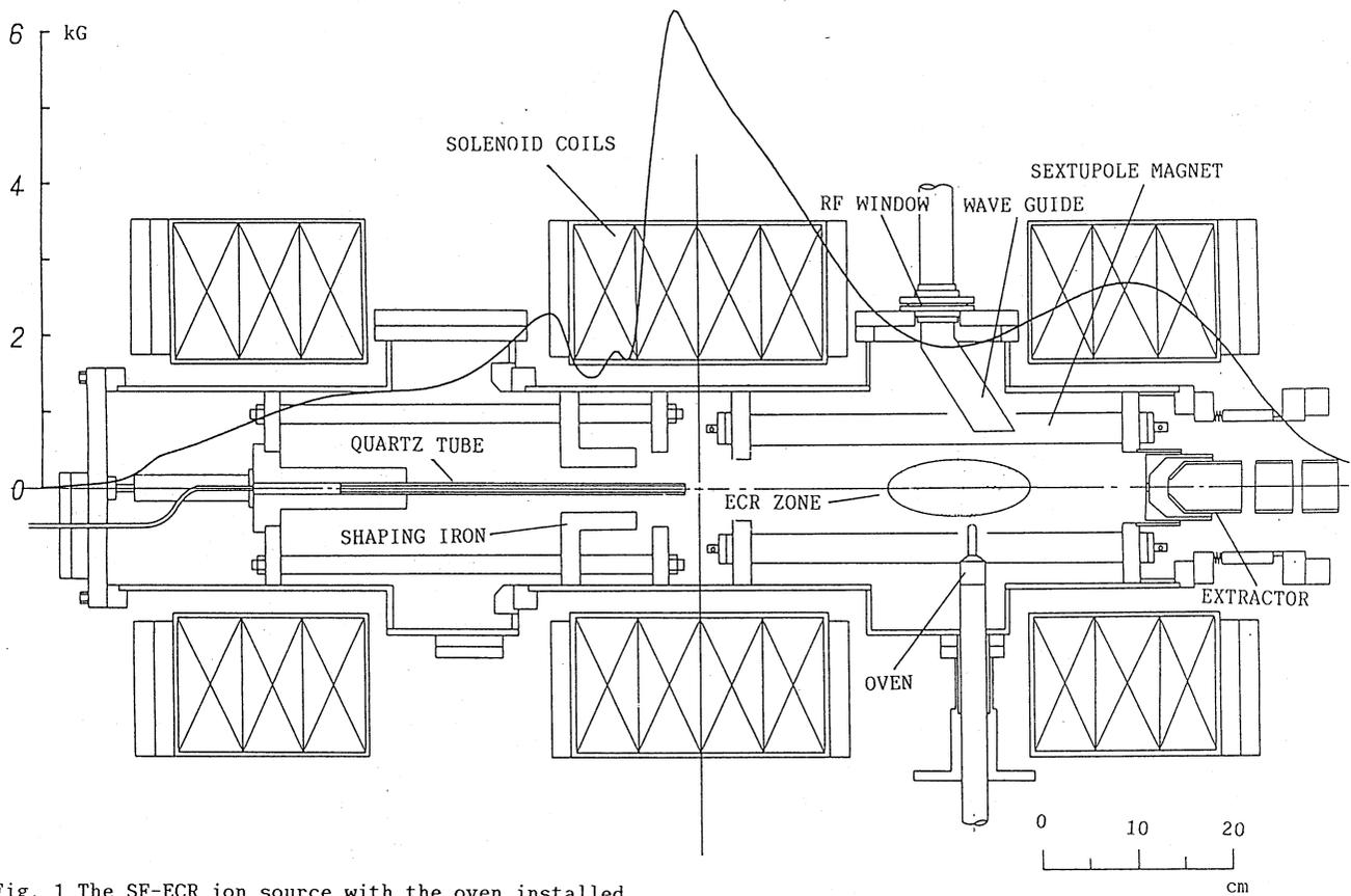
Fig. 1 The SF-ECR ion source with the oven installed and a typical magnetic field distribution during  $6\text{ Li } 2+$  beam operation.
