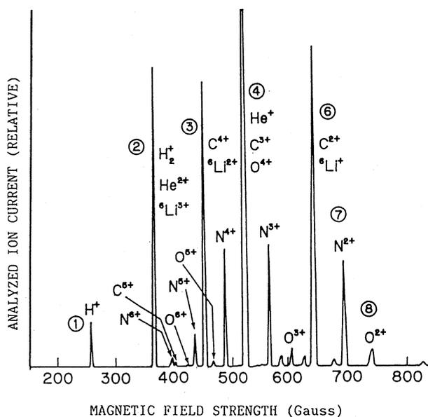
Fig. 4 A spectrum of 6 Li beam from ECR ion source tuned for 6 Li<sup>2+</sup>.
