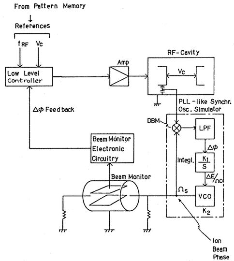
Fig. 5 Beam Simulator System ( $\Delta\Phi$  Feedback Test)
