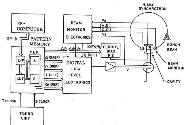
Fig. 1 RF control system of HIMAC synchrotron
