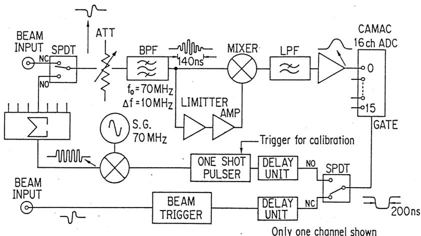
Figure 3 Detector electronics of beam position monitor.
