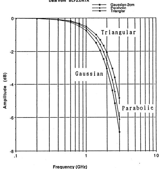
Figure 5 Beam spectra with different bunch shapes at FWBL = 8 cm.
