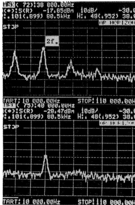
Figure 4 Coherent oscillations at higher(a) and lower(b) bunch lengths between the jumps at beam current of 4mA and  $V_c=1.18$  MV.
