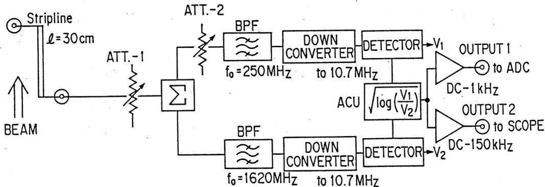
Figure 1 Simplified block diagram of bunch length monitor.
