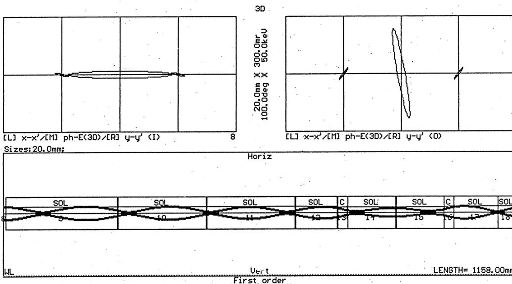
Fig. 4 Beam envelope of low current mode.
