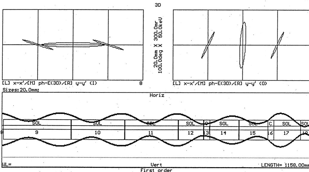
Fig. 3 Beam envelope of high current mode.
