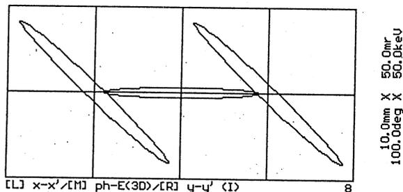
Fig.1 Initial beam ellipse of high current mode.
