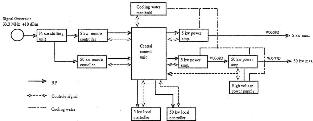
Fig.4. Block diagram of 33.3 MHz RF P.A. system.
