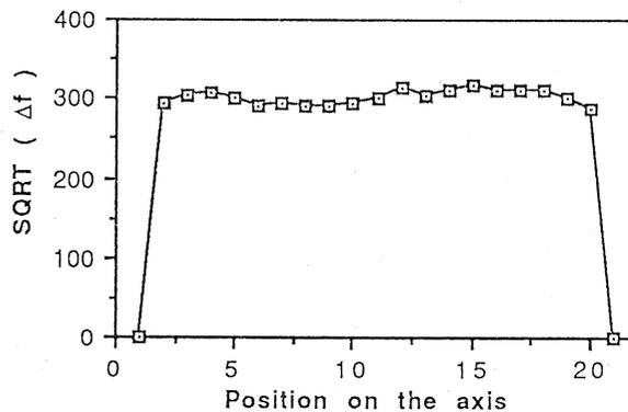
Fig. 2. Typical on-axis electric field distribution of 4-rod RFQ 1/3 scale cold-model. The resonant frequency is 94.72 MHz.
