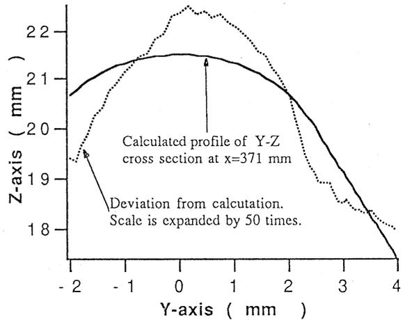
Fig. 3. Cross section plot of 1/3 scale RFQ electrode of calculated and measured profile. Dotted plot shows deviations from the calculation, brew up in scale by 50 times.
