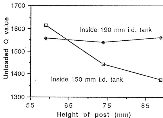
Fig.1. Unloaded Q-value as a function of post height.
