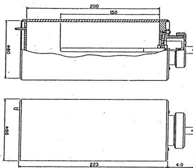
Fig. 1. Structure of cylindrical chamber cell
