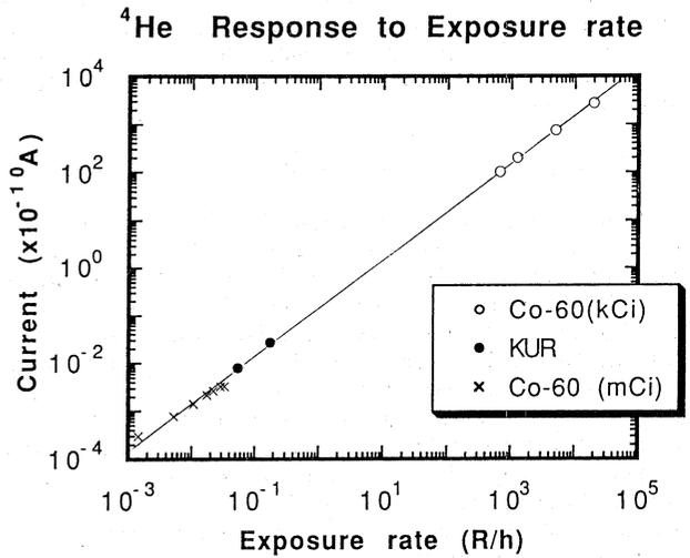
Fig. 5. Current from <sup>4</sup>He chamber vs. exposure rate
