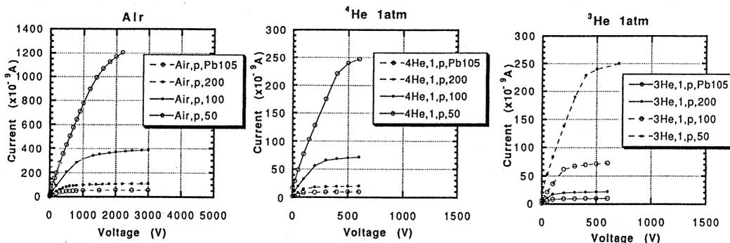
Fig. 2. Ionization chamber saturation curves (outward positive potentials)
