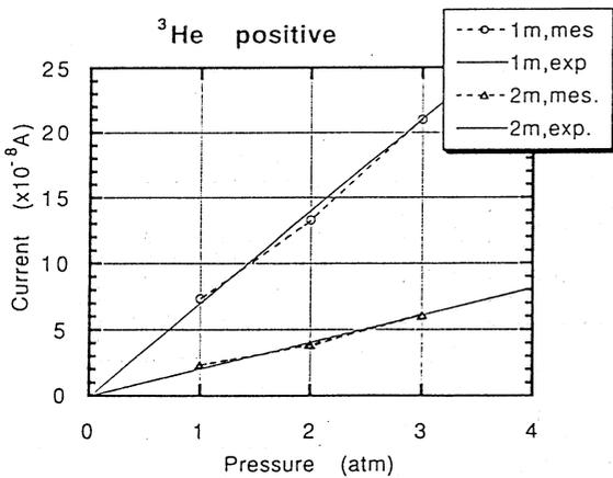
Fig. 4. Saturation current vs. gas pressure
