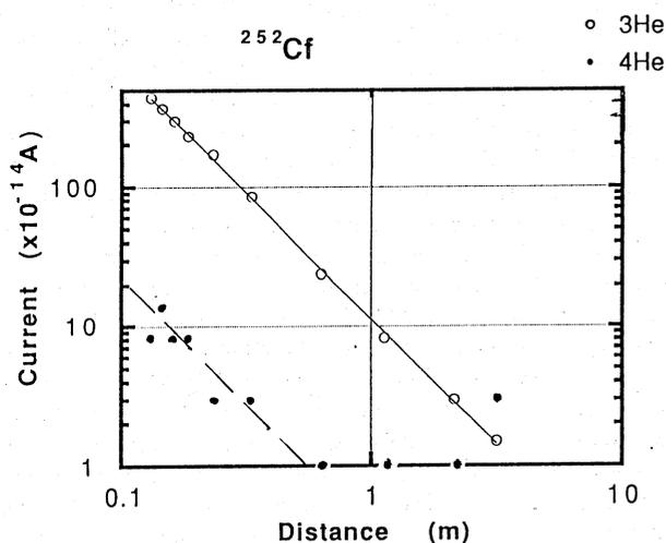
Fig. 7. Chamber responses in <sup>252</sup>Cf field versus source distance
