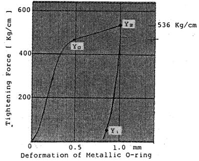
Fig. 6, The characteristic curve of stress-deformation of the Helicoflex
