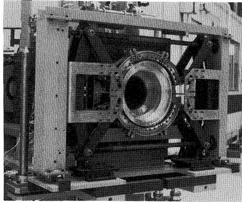
Fig. 7, The structure of the vacuum flange disconnect system.
