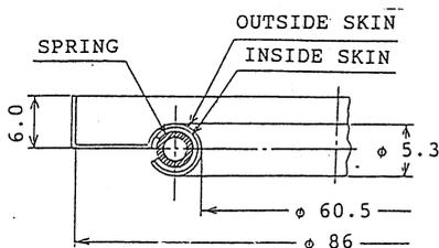
Fig. 5, The cross sectional view of a metal gasket (Helicoflex)
