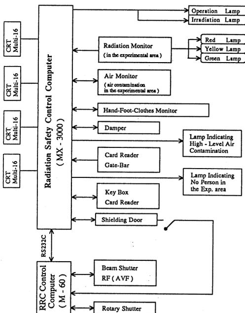
Fig.2. Block diagram of the Radiation protection control system
