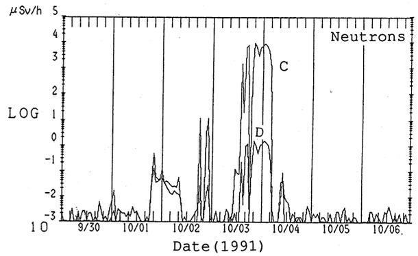
Fig.1. Comparison of day variations of the radiation level measured with radiation monitors in the E1, and E2 experimental rooms. A:  $\gamma$ -rays in E1 room, B:  $\gamma$ -rays in E2 room, C: neutrons in E1 room, D: neutrons in E2 room.
