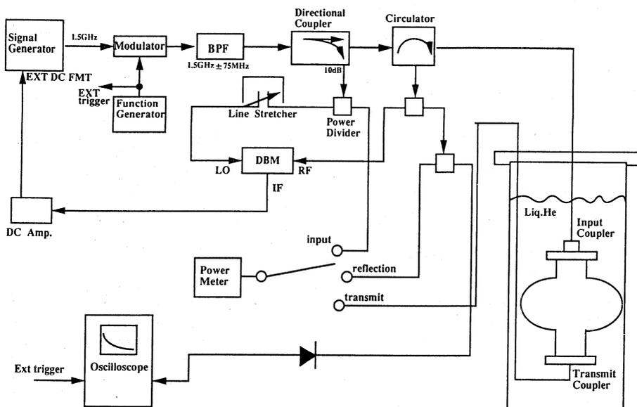
Fig.3 Measurement circuit of Q-values
