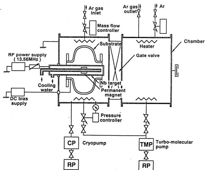
Fig.1 RF magnetron sputtering system
