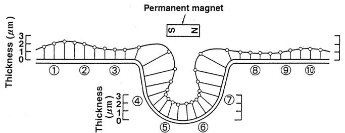
Fig.2 Thickness of niobium film on 1.5GHz single cell cavity
