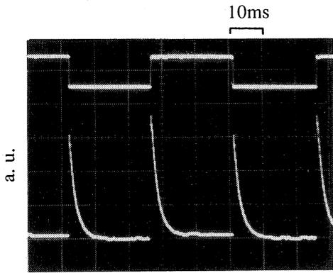
Fig.4 Input signal (upper) and reflected signal (lower)
