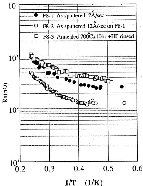
Fig.5 Dependence of surface resistance ( $R_s$ ) on temperature [1.5GHz]
