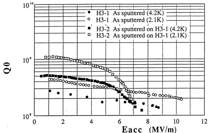
Fig.6  $Q$ -values vs accelerating fields ( $E_{acc}$ ) [1.3GHz]
