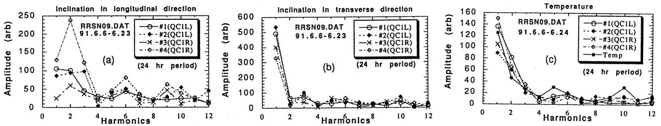
Fig.6 Harmonic components of tilt and temperature of quadrupoles of all data taken from June 6 through 23, 1991. (a) longitudinal tilt, (b) transverse tilt and (c) temperature.
