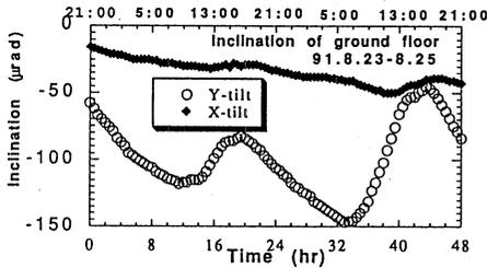
Fig.2 Inclination of the ground floor due to the variation of outdoor temperature, while the room temperature was maintained constant.
