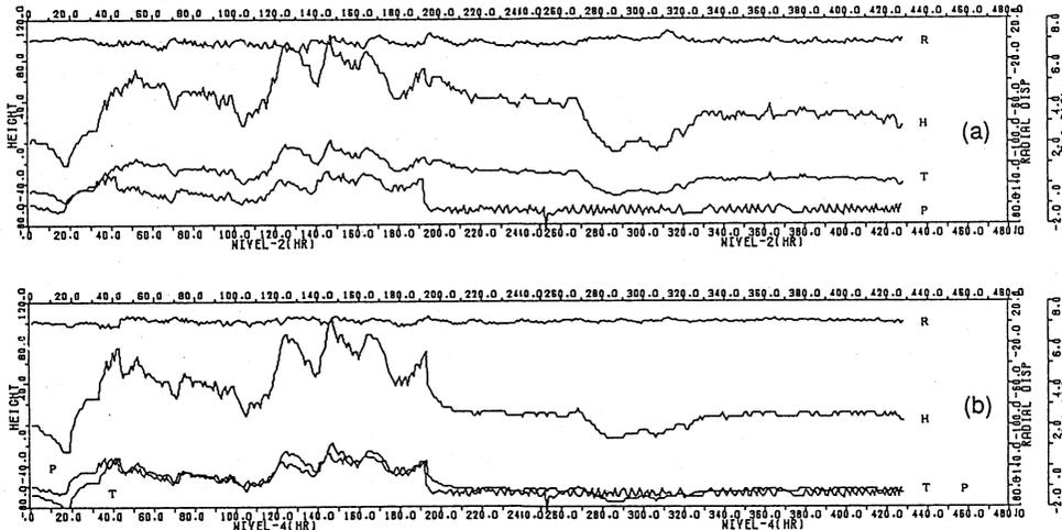
Fig.7 Horizontal displacement and vertical height variation of (a) QCS-L and (b) QC1-R. Temperature data are same as in Fig.5 and the NIVEL20 temperature is relative to that of Fig.5(a). R; radial displacement (20  $\mu\text{m}/\text{div}$ ), H; height variation (20  $\mu\text{m}/\text{div}$ ), T; NIVEL20 temperature and P; Pt thermo-sensor (1 C/div).
