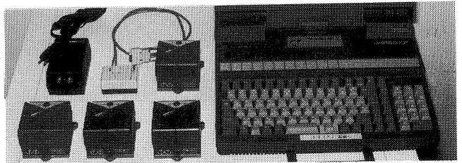
Fig.1 System of tilt meters.
