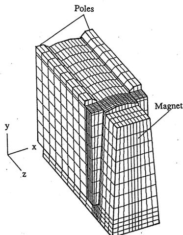
Fig.1 Three-dimensional view of the mesh reproducing a half-periodic and quarter part of the undulator.
