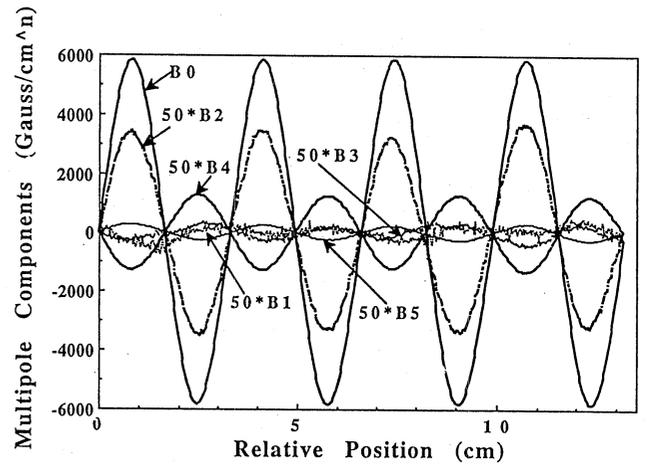
Fig.5 Longitudinal distribution of the multipoles obtained from the measured map. The higher multipoles were multiplied by fifty, to compare with others easily.
