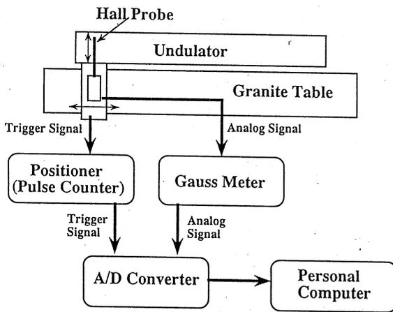
Fig.3 Schematic diagram of the measuring equipment.
