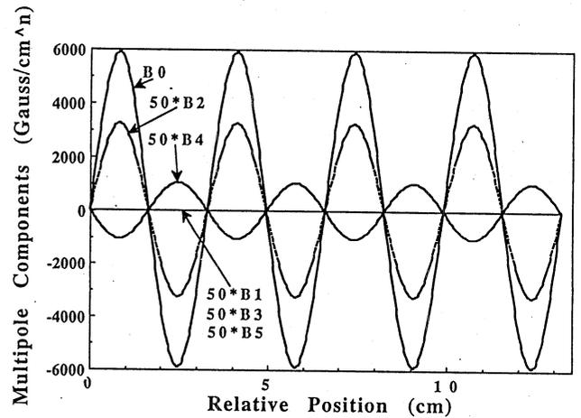
Fig.6 Longitudinal distribution of the multipoles obtained from the calculated map. The higher multipoles were multiplied by fifty, to compare with others easily.
