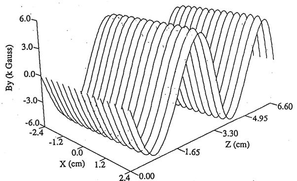
Fig.2 Calculated map in the median plane of the undulator filed.
