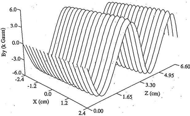
Fig.4 Measured map in the median plane of the undulator filed.
