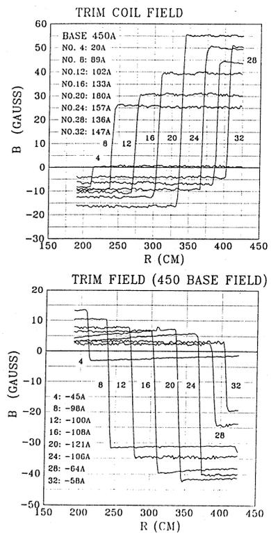
Fig. 6. Examples of trim coil field distributions along the sector center line in the case of the field gradients corresponding to the 400 MeV proton and 400 MeV alpha particle field gradients at 450A base field.
