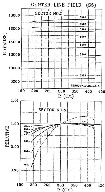
Fig. 4. The base field distributions along the center line of the No.5-sector for the main coil currents and the relative strength.
