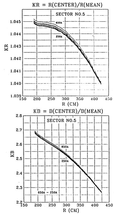
Fig. 5.  $K_b$  and  $K_r$  values of the six sectors at 500A excitation.
