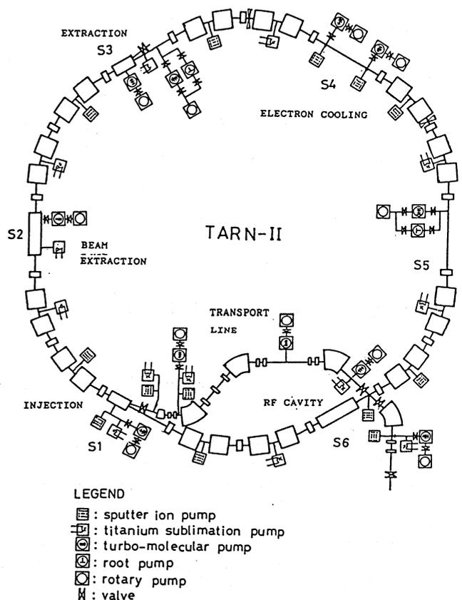
Fig.1 The vacuum system of TARN II
