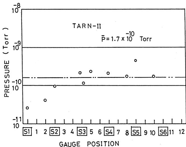
Fig. 4 The vacuum pressure measured at ten points around the ring without a beam.
