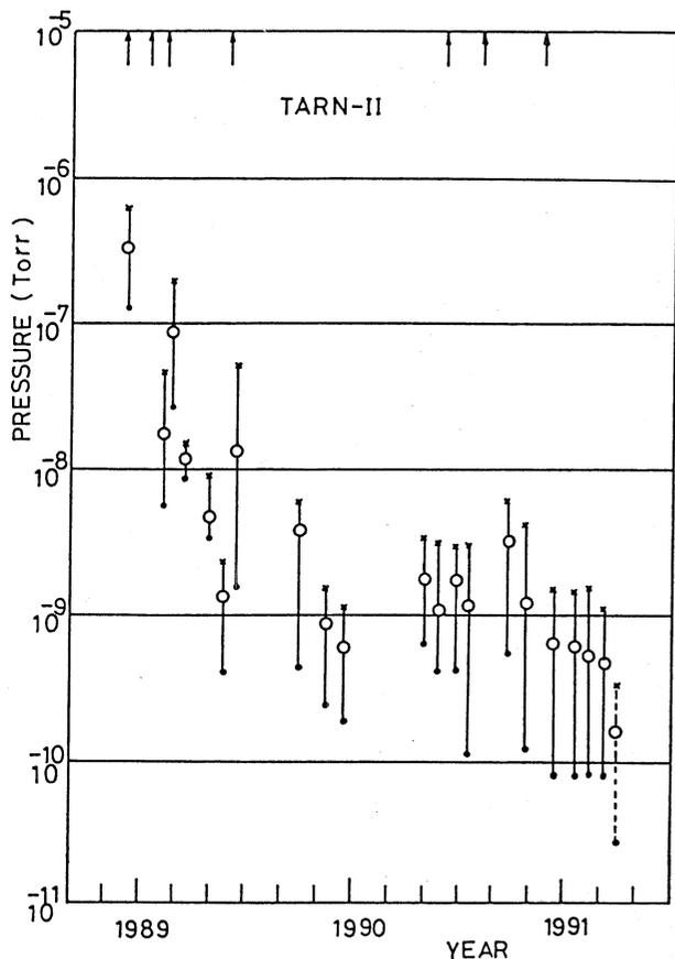
Fig.2 Mean pressures at machine times from the first beam experiments. Good and bad values at the measuring points are indicated by black dots and crosses respectively. The last point (indicated by the dotted line) is the based pressure for the condition of without a beam.
