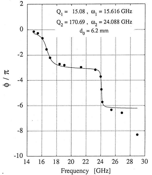
Figure 2 Phase variable  $\phi$  as a function of frequency  $\omega$  for a structure of type B with its iris opening width 8mm.
