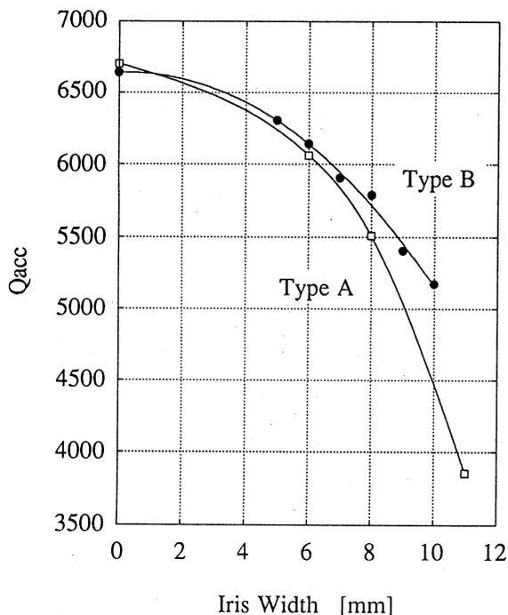
Figure 3.b  $Q_{acc}$  as a function of iris width.
