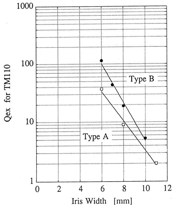
Figure 3.a  $Q_{ex}$  for TM<sub>110</sub> as a function of iris width.
