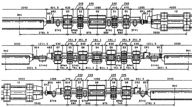
Fig. 8. Layout of magnets and vacuum components in a cell. Unit cell has two bending chambers and three straight section chambers.
