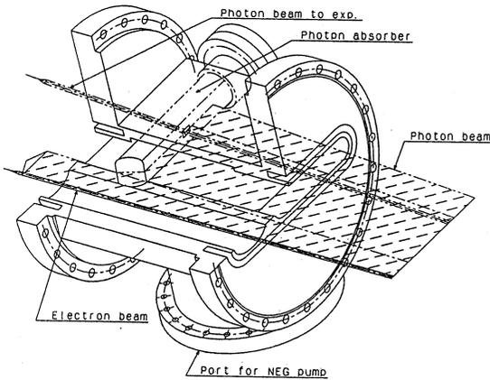
Fig. 10. Isometric view of a crotch. Most of the radiation from bending magnets are intercepted by this crotch and absorber(not indicated).
