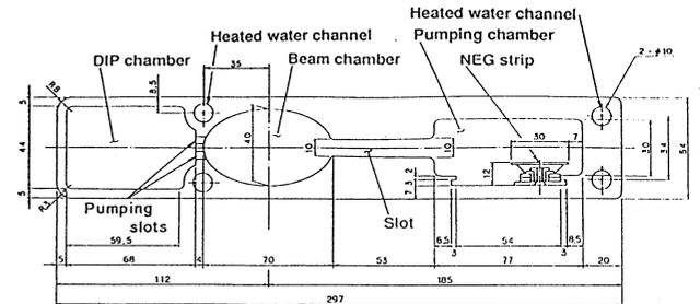
Fig. 9. Cross section of vacuum chamber. Upper is a straight section vacuum chamber and bottom is a bending section chamber. Main pump is the NEG strip attached to the antechamber part. Distributed ion pump is used for bending chamber using the magnetic field of dipole magnet.
