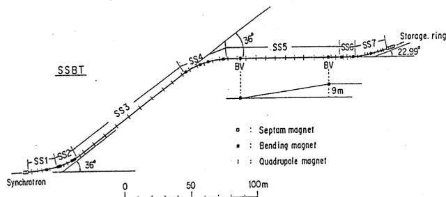
Fig.6 Beam transport from synchrotron to storage ring.
