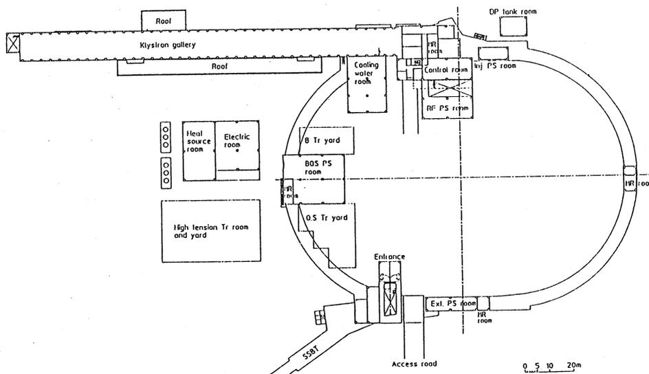
Fig.7 Buildings for injector system.
