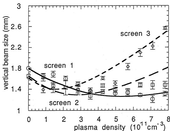
Fig. 4. Experimental and theoretical dependences of vertical beam sizes at the three screens on the plasma density.
