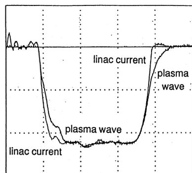
Fig. 3. Envelopes of the linac beam current and the plasma oscillation. The horizontal scale is 2μsec/div., and the vertical scale is arbitrary.
