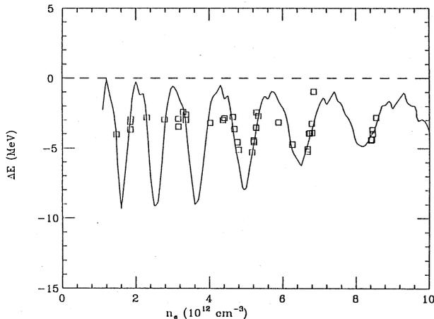
Fig. 2 Experimentally obtained energy shifts of the third bunch. The solid line shows calculated energy shifts.
