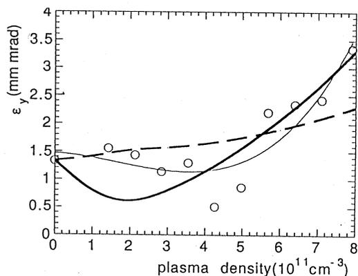
Fig. 5. Dependence of vertical emittance on plasma density. Data points and the thin solid line were calculated directly from the measured beam sizes, while the thick solid lines was calculated from the quadratic approximation of data points of Fig. 4. The dashed line was calculated based on the round-beam model.
