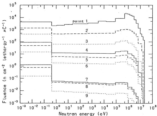
Fig.2 Neutron energy spectra measured by the Bonner Ball in the cyclotron room and the labyrinth at CYRIC.
