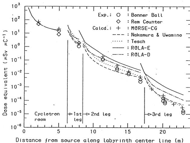
Fig.3 Dose equivalent distribution measured by the Bonner Ball and the rem counter compared with five different calculations (four simple formulas and the MORSE-CG).
