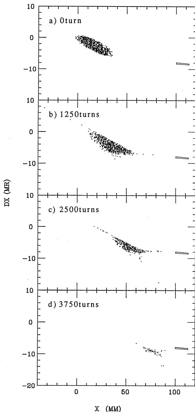
Fig. 4 Results of multi-particle tracking. All particles are extracted through the solid box in these figures. Figures (a)-(d) show the particles after 0, 1250, 2500, 3750 turns, respectively.
