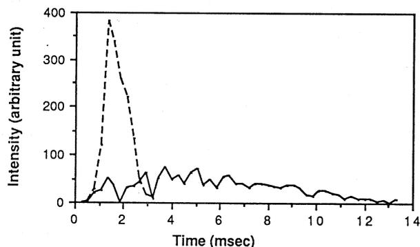
Fig.5. Calculated time structures of the beam spill.
