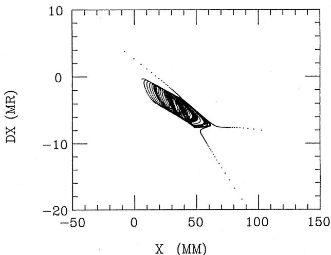
Fig. 2 The motion of a particle in the horizontal phase space. The electric septum is located at the position apart from the designed orbit by 100mm.
