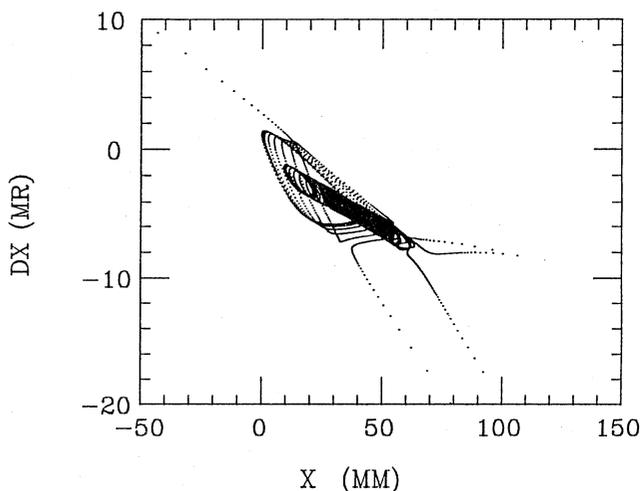
Fig. 3 An example of overlapping of outgoing separatrices between two particles with different amplitude.
