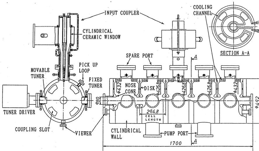
Figure 1. Cross sectional view of the prototype cavity
