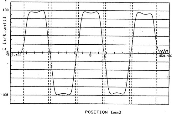
Figure 4. Field distribution of the accelerating mode
