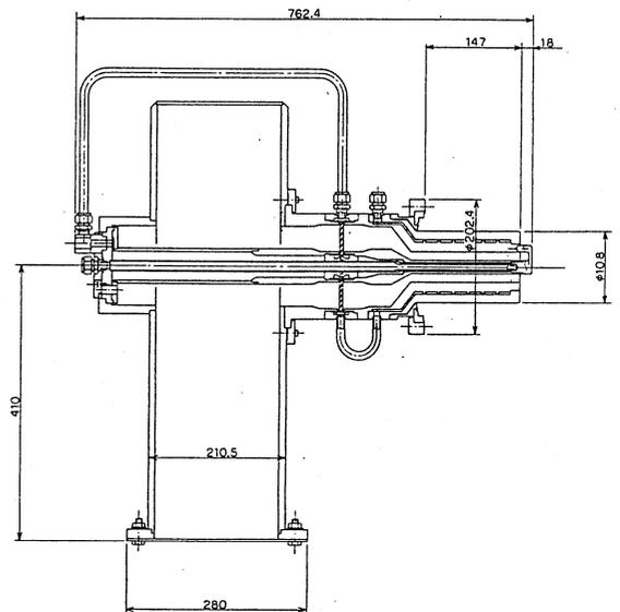
Figure 3. Input coupler with the disk type window
