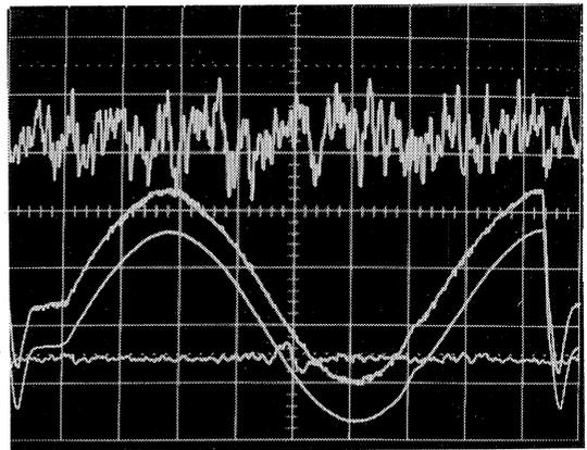
Fig. 6 Beam phase profile measured with phase probe for 50 nA beam. The beam signals from the probe were measured with a sampling oscilloscope and averaged 100 times with digital oscilloscope.
