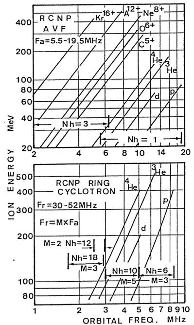
Fig. 4 Orbital frequencies, acceleration frequencies and harmonic numbers of acceleration in the AVF cyclotron and the RCNP ring cyclotron. M is ratio of the RF frequency of the ring cyclotron to the AVF cyclotron.
