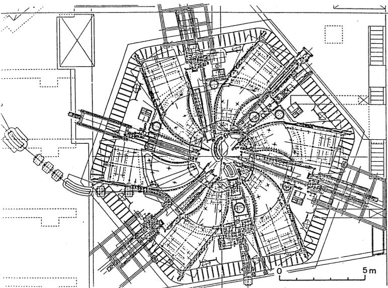
Fig. 3 Plan view of the ring cyclotron.
