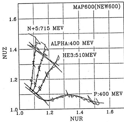
Fig. 5 Comparison between betatron frequencies calculated from the measured field and the designed one.
