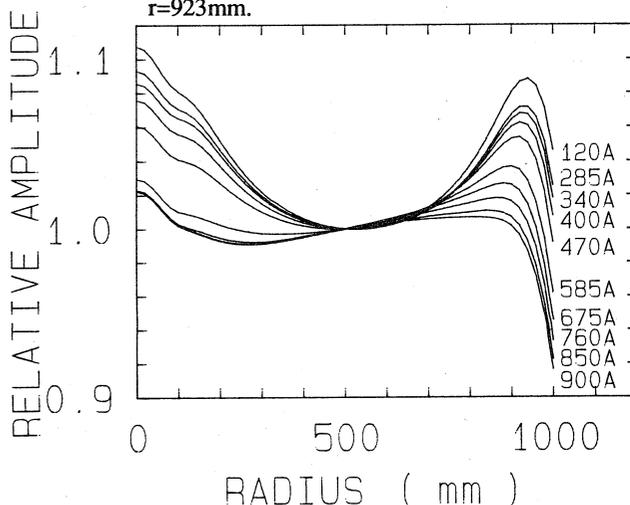
Fig. 3 Radial distributions of the main coil field at ten field levels. The field strength is expressed in relative amplitude to the strength at  $r=500\text{mm}$ .
