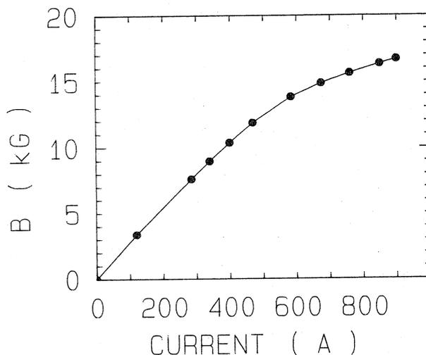
Fig. 2 Excitation curve at an extraction radius of  $r=923\text{mm}$ .
