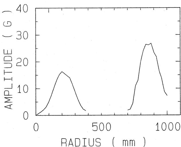
Fig. 6 First harmonic amplitude generated by two pairs of harmonic coils placed in a central and an extraction regions.
