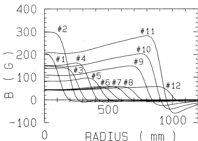
Fig. 5 Radial distributions of twelve trim coil fields at a base field level of 585A.
