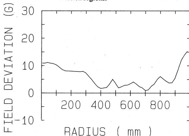
Fig. 7 Difference between the calculated isochronous field and the measured field for 75 MeV proton. The calculated field is produced by the optimization calculation based on the measured main and trim coil field maps.
