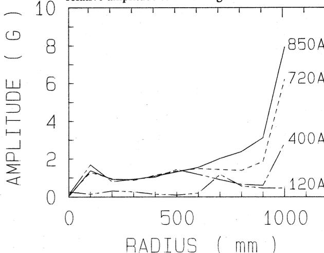
Fig. 4 First harmonic amplitude versus radius for four base field levels of 120A, 400A, 720A and 850A.
