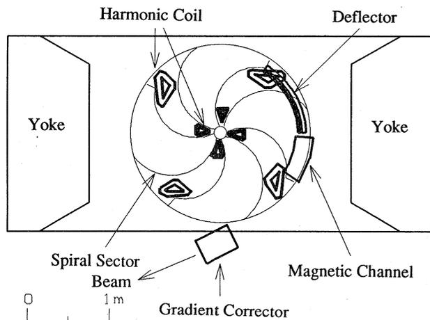
Fig. 1 Schematic view of the JAERI AVF cyclotron.
