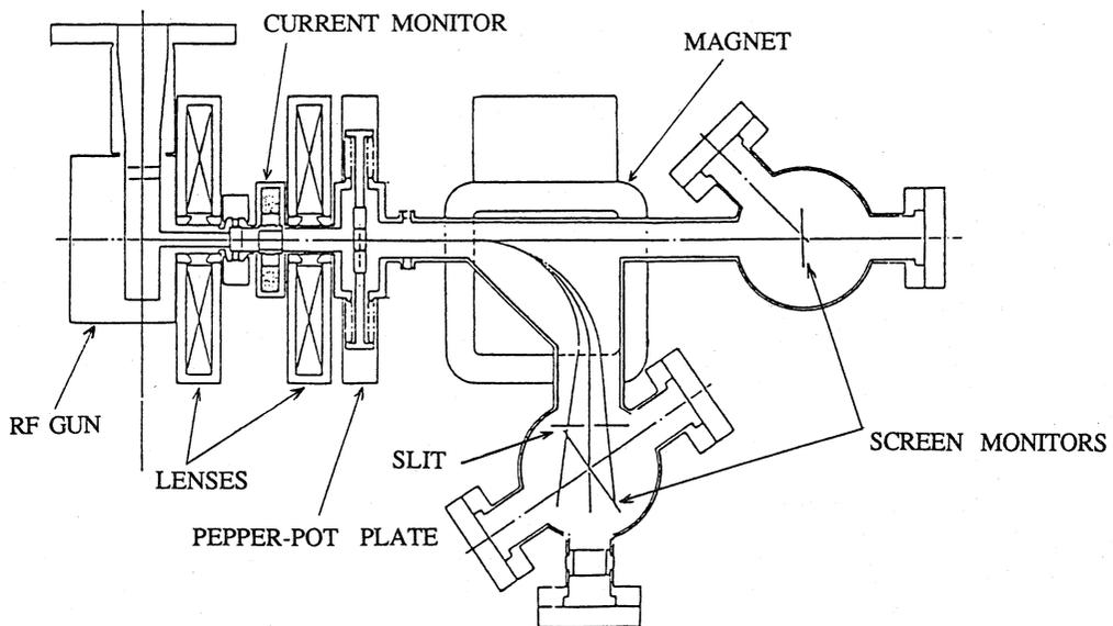
Fig.3 Composition of the test bench.
