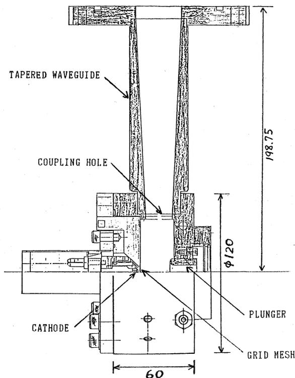
Fig.1 Cross-sectional view of the cavity.
