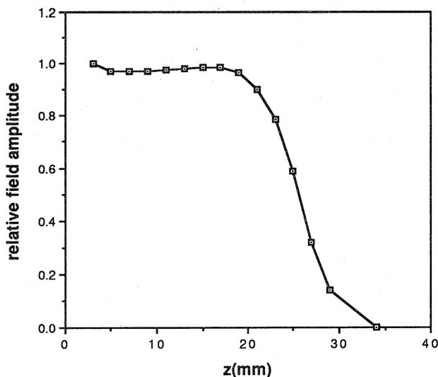
Fig.2 Measured electric field profile along the beam center line of the cavity without a mesh grid.
