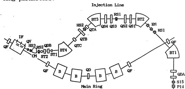
Fig. 2 Transport and injection line in the TARN II room. See the text for each element.
