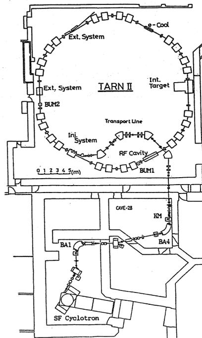
Fig. 1 Layout of SF Cyclotron and TARN II.
