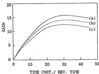
Fig. 4 Gain of multi-turn injection versus damping time constant of bump field.
