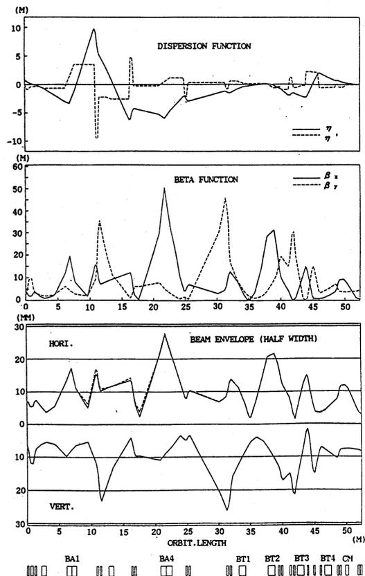
Fig. 3(a) Dispersion function  $\eta$  and its derivative  $\eta'$  and beta functions  $\beta_x, \beta_y$ .
