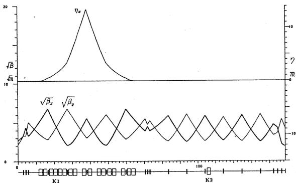
Fig.3. The betatron and dispersion functions at the  $H^-$  injection line.  $\eta_x$  is the horizontal dispersion function.  $\sqrt{\beta_x}$  and  $\sqrt{\beta_y}$  are square roots of the horizontal and vertical betatron functions, respectively.
