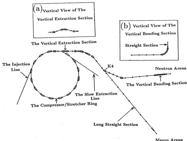
Fig.6. The fast extraction line to Meson and Neutron Arenas. The box denoted by (a) and (b) show the vertical views of the vertical extraction section from the ring and of the vertical bending section under Neutron Arena, respectively.
