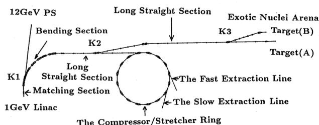
Fig.2. The beam transport line from the 1GeV linac.
