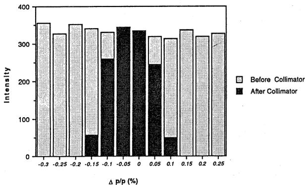
Fig.4. The result of scraping the momentum halo by the scraper at the center of bending section(Fig.2). The beam of  $\epsilon_x = 1.2\pi mm \cdot mrad$ ,  $\epsilon_y = 1.4\pi mm \cdot mrad$  and  $\Delta p/p = 0.3\%$  can be scraped as  $\Delta p/p = 0.1\%$ .
