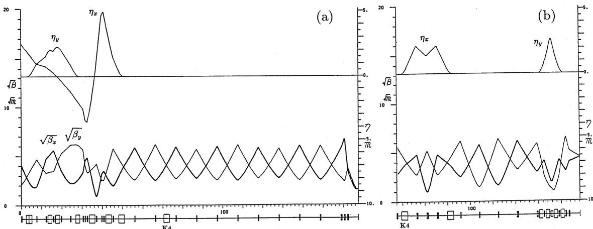
Fig.7. The betatron and dispersion functions of the fast extraction line to Meson Arena (Fig.7-a) and to Neutron Arena (Fig.7-b). The long straight section and the straight section near the target of Neutron Arena are dispersionless.
