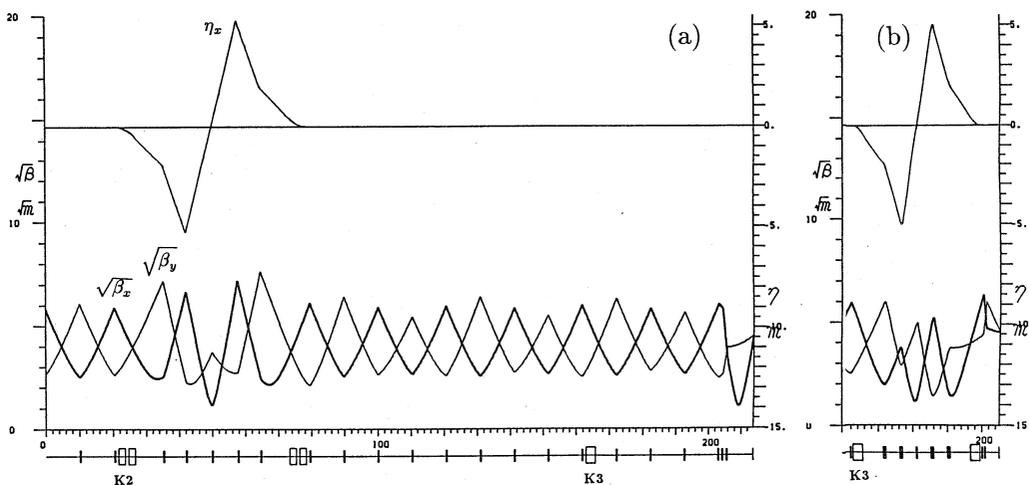
Fig.5. The betatron and dispersion functions at the transport line to Exotic Nuclei Arena. Figure 5-a shows the functions between K2 magnet and the target(A) of Exotic Nuclei Arena. Figure 5-b also shows the functions between K3 magnet and target(B).
