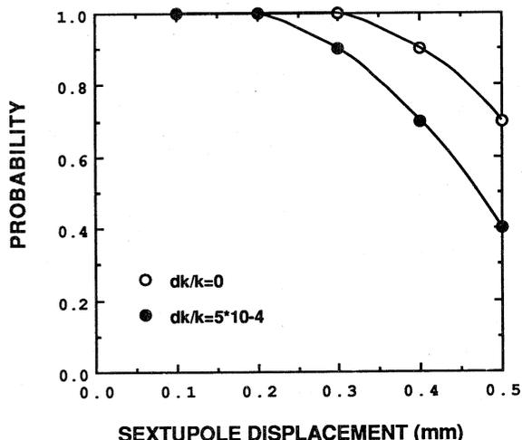
Fig. 3 Effects of sextupole displacements and quadrupole gradient errors on stability of betatron oscillation
