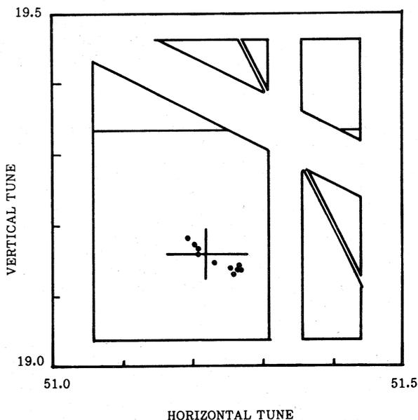
Fig. 5 Stopbands of lowest-order accidental sum resonances and tune shift ( $2\sigma$ )
