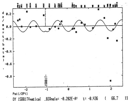
Figure 2: The measured (squares) and the calculated (curve) beam positions of the corrector with the least significant secondary kick.
