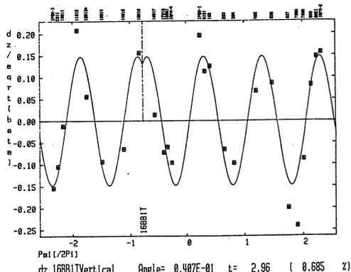
Figure 1: The measured (squares) and the calculated (curve) beam positions of the corrector with the most significant secondary kick.
