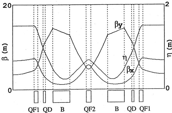
Fig.2 Lattice functions in operation
