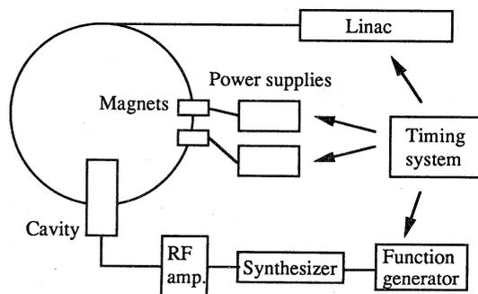
Fig.5 Block diagram of RF frequency modulation system
