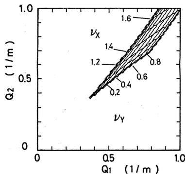
Fig.6 Tune diagram of the dispersion free operation of DBA
