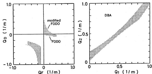
Fig.4 Tune diagrams for FODO, modified FODO, and DBA
