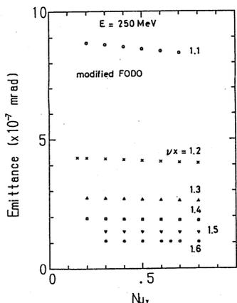
Fig.7 A plot of the beam emittance as a function of betatron tune for DBA
