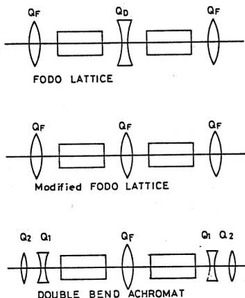
Fig.3 Types of magnetic lattices
