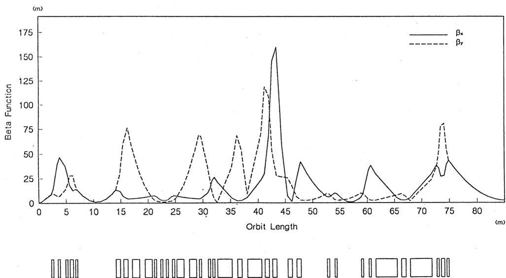
Fig. 3. Beta function of the vertical beam transport line to the iso-center of the treatment room B.
