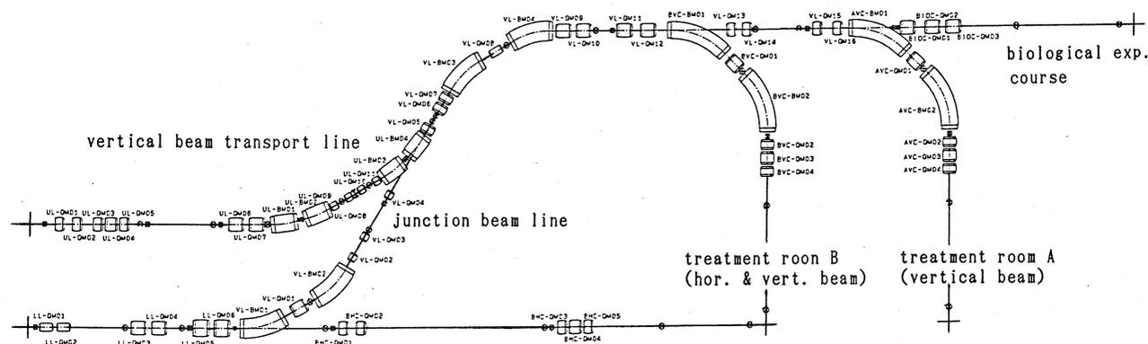
Fig. 2. A side view of the vertical beam transport line.
