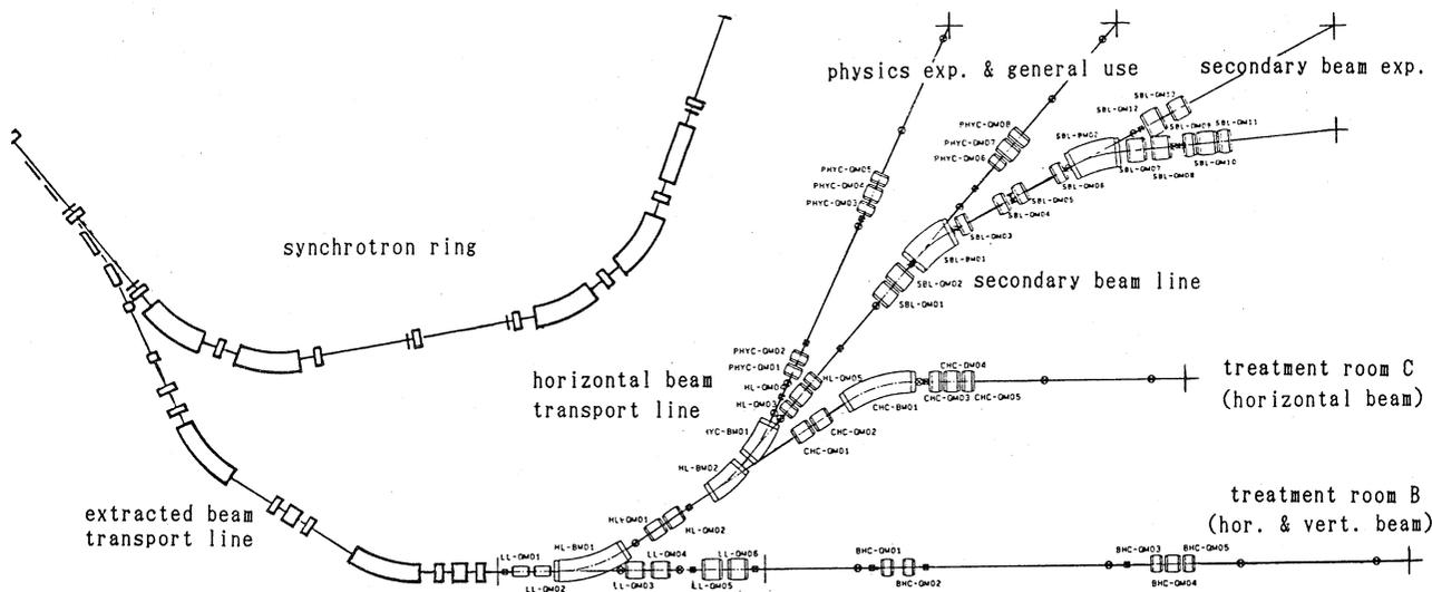
Fig. 1. A plan view of the extracted and the horizontal beam transport line.
