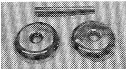
Fig. 2. Drift tube end plates and a bore tube.
