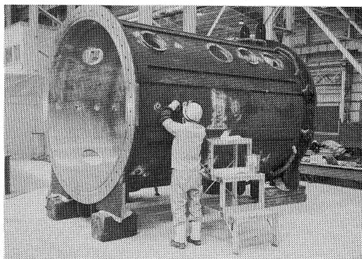
Fig. 1. Alvarez no.3 tank under machining.
