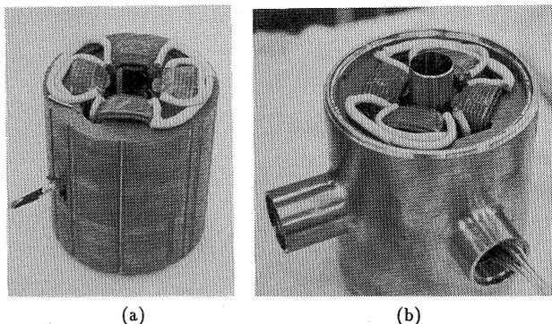
Fig. 3. A quadrupole magnet before (a) and after (b) assembling.
