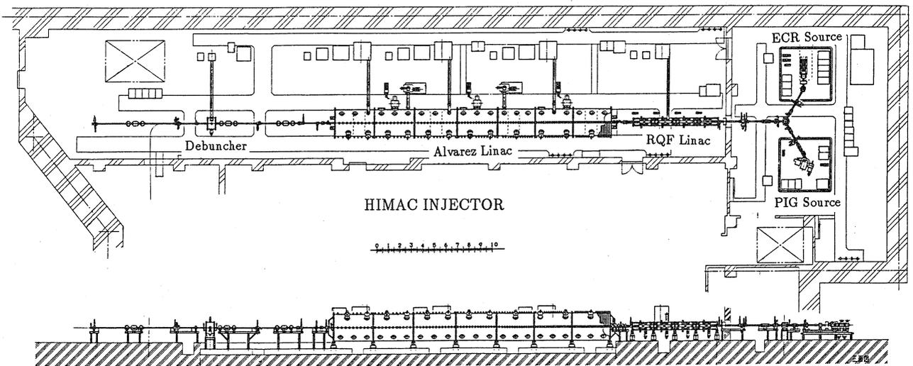
Fig. 4. A layout of the HIMAC injector.
