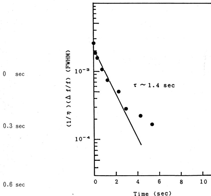
Fig. 3 Time dependence of the frequency spread of 38th harmonic of beam signal.
