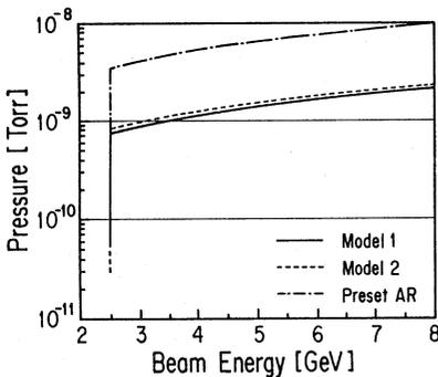
Fig.4 Calculated pressure in the beam duct for each DIP.
