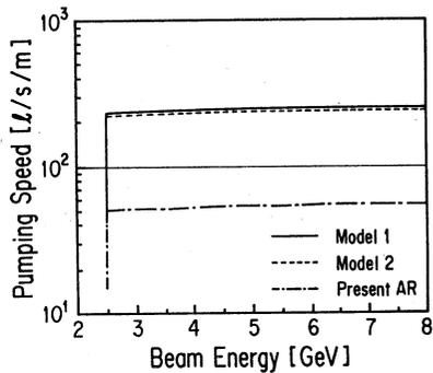
Fig.3 Calculated pumping speed for each DIP.
