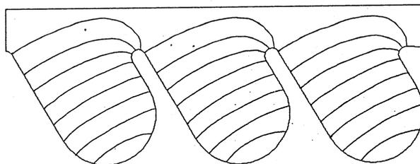
Fig.2 Side view of the electric focusing structure. Bunches travel from left to right.
