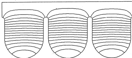
Fig.1 Side view of conventional structure of DAW. This is modified type for high shunt impedance at SLAC.
