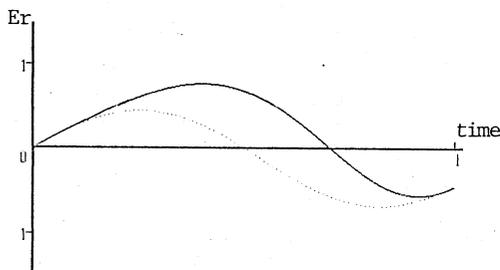
Fig.6 Radial component of electric field, which received by a synchronous particle as  $\beta=0.85$ .
