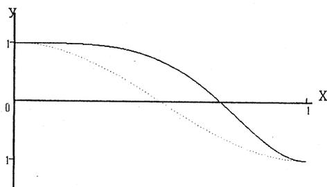
Fig.4  $y = \cos(\pi X^2)$  is shown as a line, and  $y = \cos(\pi X)$  is shown as a dotted line.  $X = x/D$ , D:axial length of one cell.
