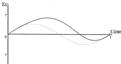
Fig.5 Radial component of electric field, which received by a synchronous particle as  $\beta=1$ . The dotted line shows radial component of conventional DAW.
