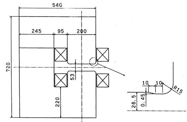
Fig. 4 Cross section of the dipole.
