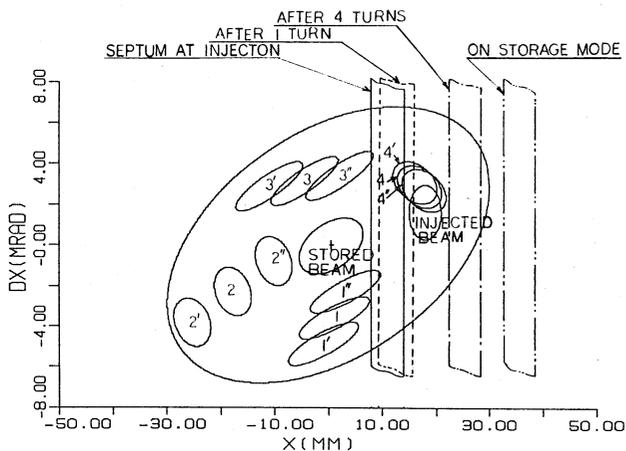
Fig. 3 Motions of injected and stored beams at the exit of the inflector.
