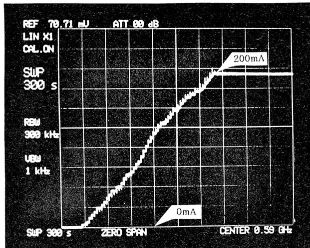
Fig. 10 Beam current during the injection.
