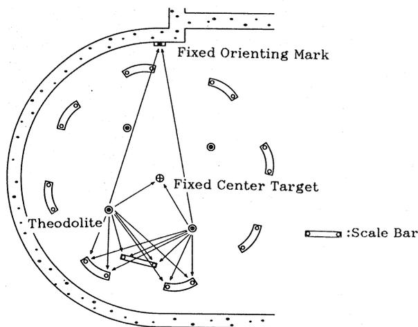
Fig. 6 Surveying procedure for the horizontal alignment of the dipoles. The instrument is rotated by  $90^\circ$  in turn for alignment of every two neighboring dipoles.
