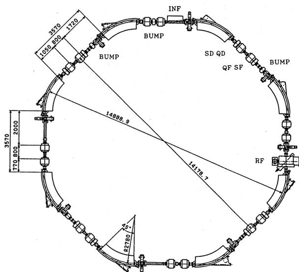
Fig. 1 Layout of the ring.
