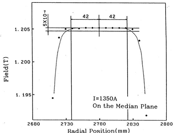
Fig. 5 Field of the dipole in the radial direction. The points mean the measured field, and the dotted line the calculated one. The pole center is at 2780mm.
