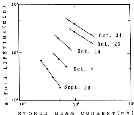
Fig. 11 History of the beam lifetime. The ion clearing has been carried out since Oct. 23.
