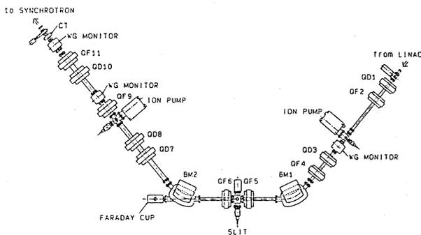
Figure 6 The layout of low energy beam transport line
