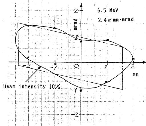
Figure 5 Emittance of buncher output
