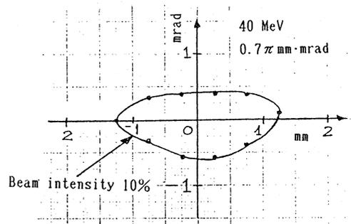
Figure 4 Emittance of linac output
