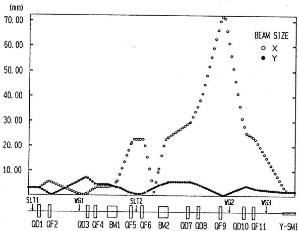
Figure 7 The beam size
