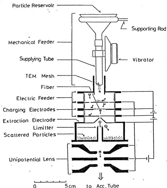
Fig.6 The fiber type macron source used on a electron Van de Graaff accelerator addition of mechanical and electrical particle feeders enabled long time operation.
