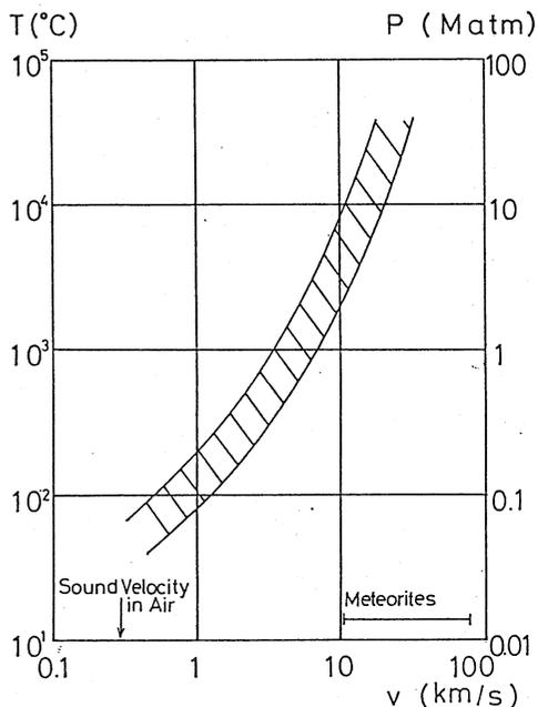
Fig.1 Variation of shock pressure and temperature with collision velocity.
