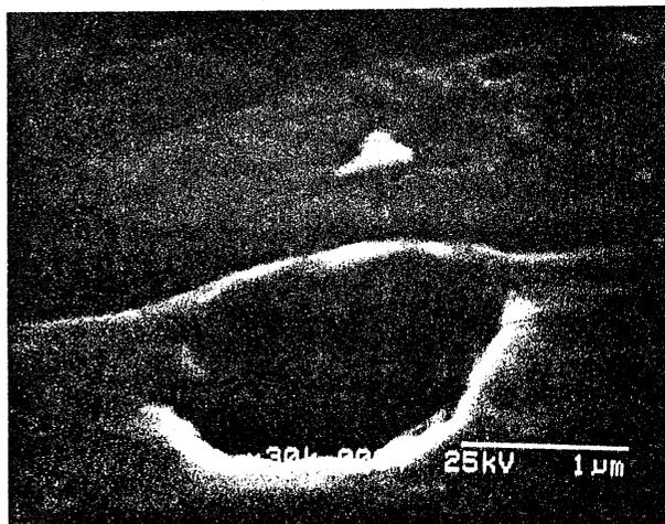
Fig.7 Microparticles produced on Cu plate bombarded by 2MV-accelerated nickel SEM angle  $60^\circ$ .
