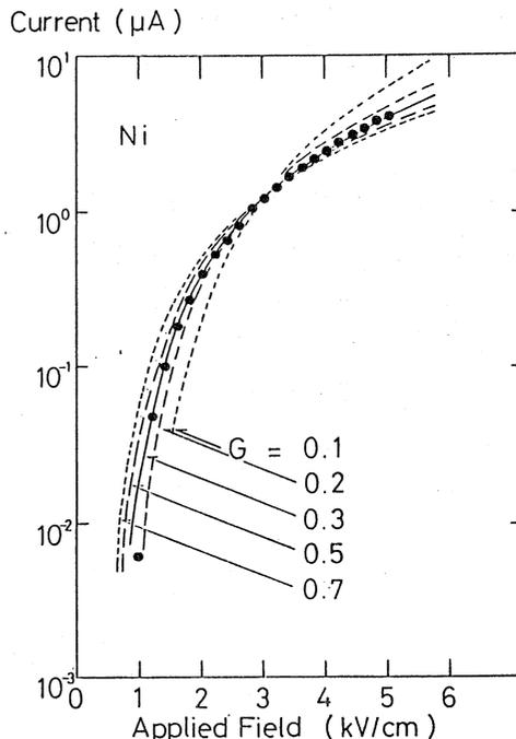
Fig.3 V-I relation of a parallel plate nickel macron source.
