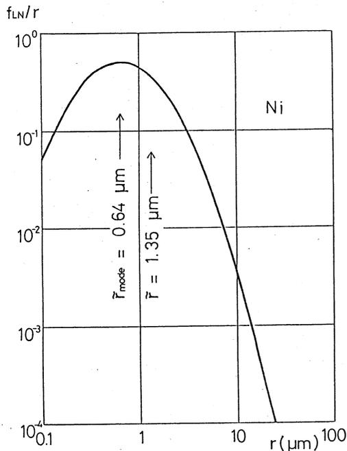
Fig.2 Size Distribution of nickel powder as the sphere of radius  $r$ .
