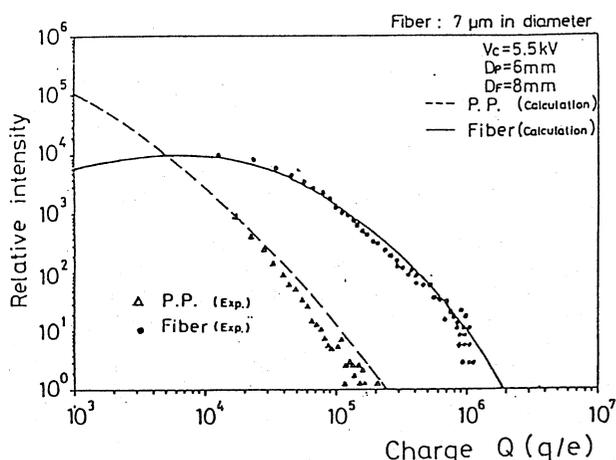
Fig.5 Charge distributions of macrons from a parallel plate type (p.p.) and fiber type (Fiber) sources.
