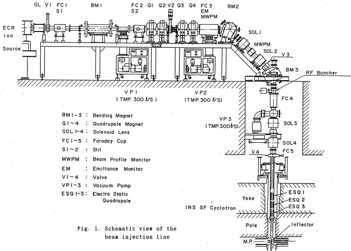
Fig. 1. Schematic view of the beam injection line
