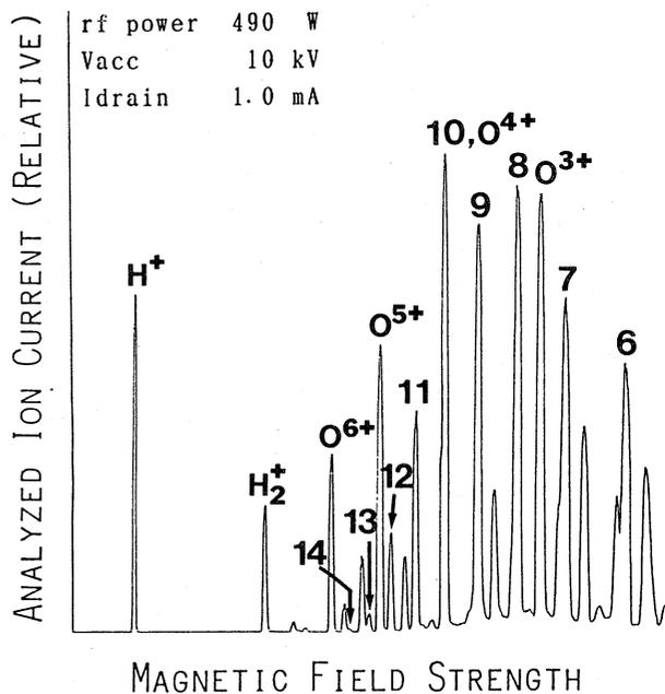
Fig. 4. A spectrum of Ar beam from ECR ion source, tuned for  $\text{Ar}^{11+}$
