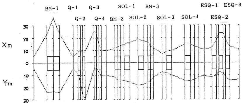
Fig. 2. Beam envelope along the injection line. calculated  $20\text{Ne}^{6+}$  beam;  $B\rho = 26\text{kG} \cdot \text{cm}$ .
