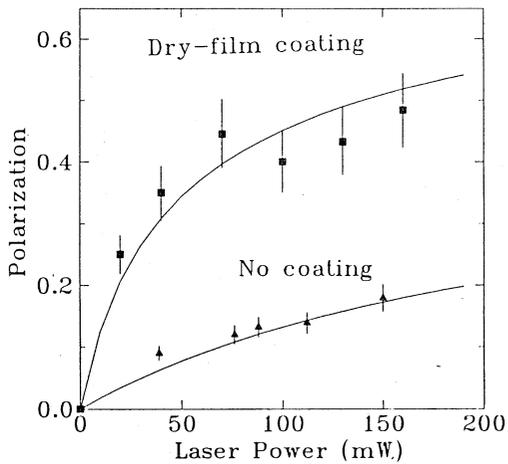
Fig.3 a) Observed polarization as a function of the pumping light intensity.
