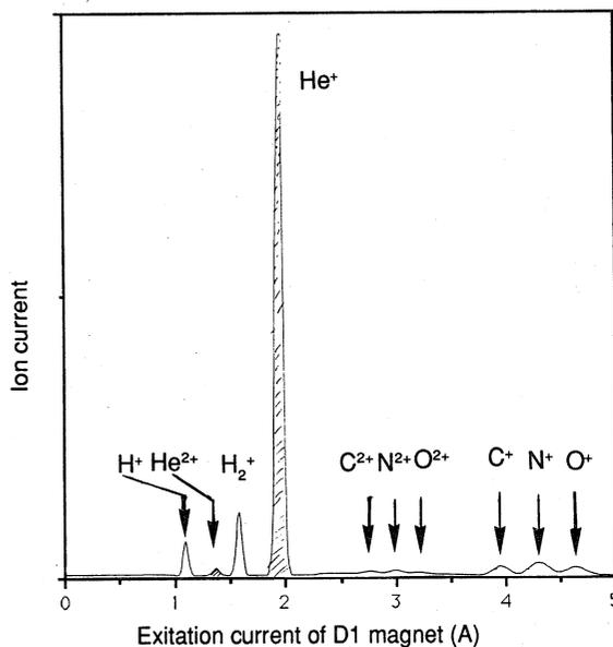
Fig.2. Ion currents measured by varying the strength of the analyzing magnet.
