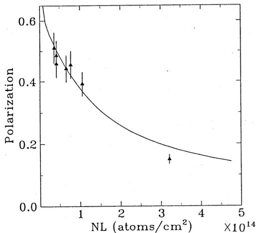
Fig.4 Observed polarization as a function of the sodium thickness.
