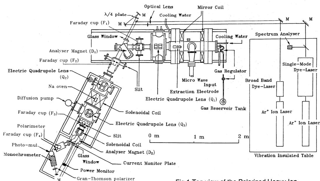
Fig.1 Top view of the Polarized Heavy Ion
