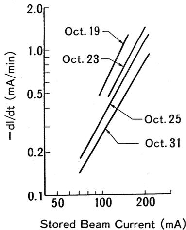
Fig. 6 The Improvement of the Beam Lifetime ( The Decay Rate Plot)
