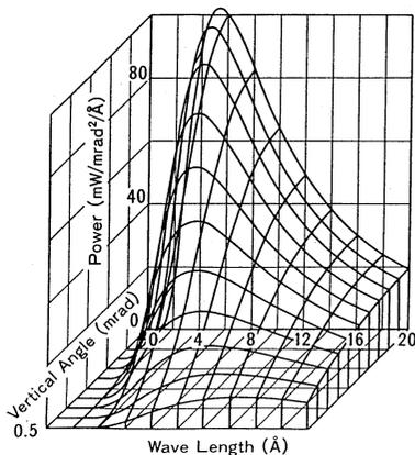
Fig. 3 Spectrum and Spatial Distribution of Synchrotron Radiation
