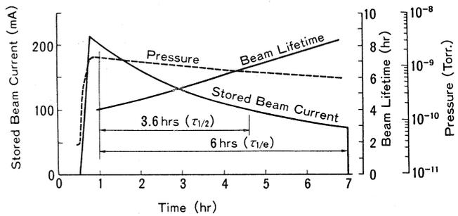
Fig. 5 Stored Beam Current, Beam Lifetime and Vacuum Pressure Obtained at the End of October 1989
