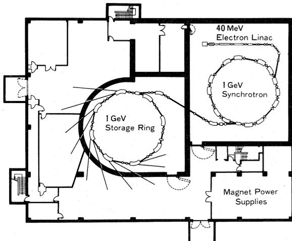
Fig. 1 Layout of the Synchrotron Radiation Source Facility
