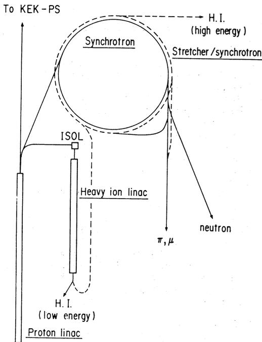
Fig. 1 Layout of the JHF accelerators.
