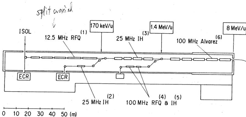
Fig. 3 Scheme of the heavy ion linacs.
