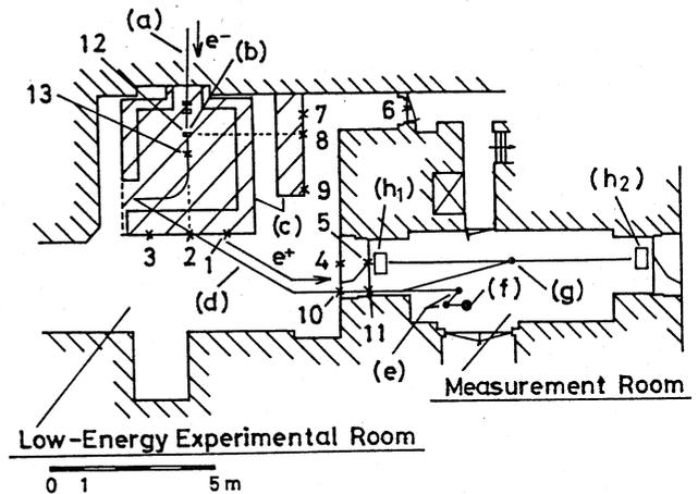
Fig. 1. Plan view of the ETL slow-positron facility.
