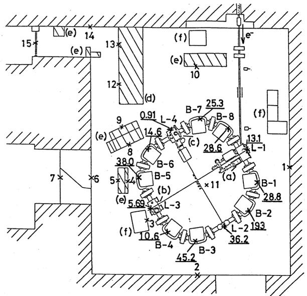
Fig. 3. Plan view of the Medium-Energy Experimental Room. Underlined figures mean integrated radiation doses caused by stored electrons in units of mR for an extraordinary case (see text).
