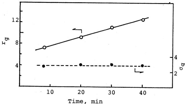
Fig. 4. Time variations of the geometric mean radius ( $r_g$ ) and the geometric standard deviation ( $\sigma_g$ ) of the aerosol particles
