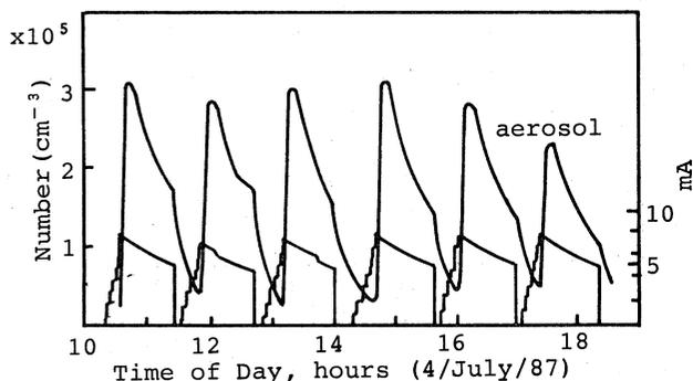
Fig. 2. Time profiles of aerosol number concentration and beam current
