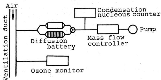
Fig. 1. Schematic diagram of Measurements
