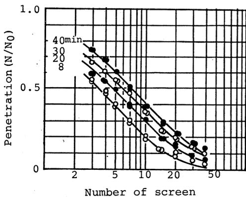
Fig. 3. Penetration of the aerosol particles produced by synchrotron radiation through the screen type diffusion battery
