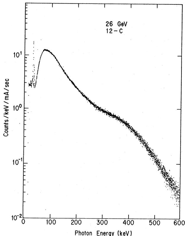
Fig. 4 Photon Energy Spectrum on the Earth's Surface Measured using HP-Ge Detector.
